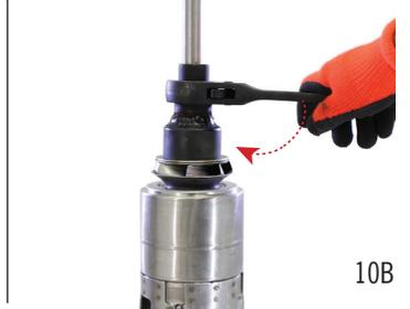
Use **TORQUE TESTING NUT** and **WRENCH** to tight at correct torque (clockwise) (Step 7)
