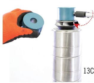
**14 Loosen with Allen Tool, remove from Fixture Seat. Remove 6" Jig with Allen Tool from Assembly**
