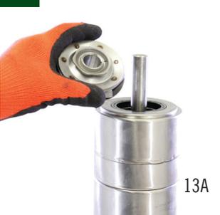
Use **WRENCH FOR IMPELLER NUT** to tighten (clockwise)
