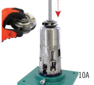
Use **WRENCH FOR IMPELLER NUT TOOL** to tighten (clockwise)
